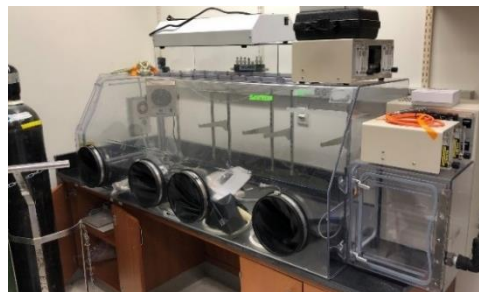
Figure 5.1: The chamber used to control the sO 2 values of the blood samples
